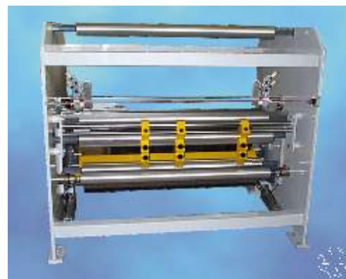
For optimum film tension control the MSG is available with integrated auxiliary nip or external secondary nip
